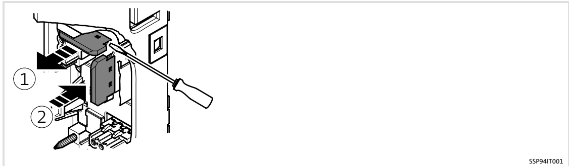
Fig. 4-19 Plugging the IT insulating cap onto the earthing jumper
