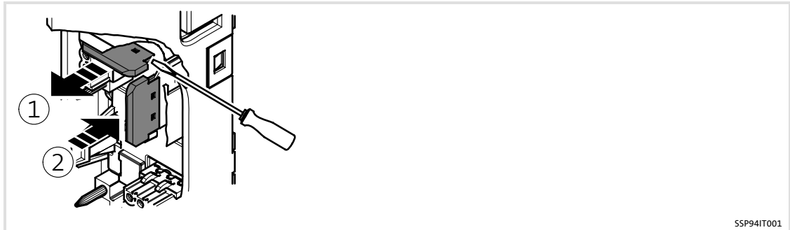
Fig. 6-5 Plugging the IT insulating cap onto the earthing jumper
